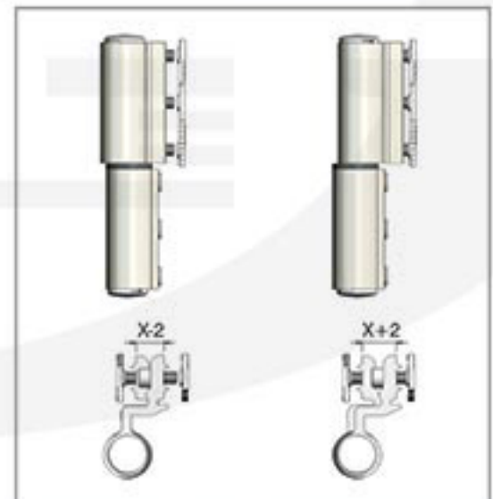
Side adjustment typical of conventional clamp-fixed hinges
