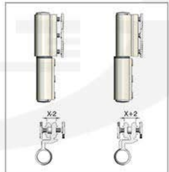
Side adjustment typical of conventional clamp-fixed hinges
