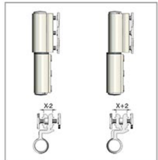
Side adjustment typical of conventional clamp-fixed hinges
